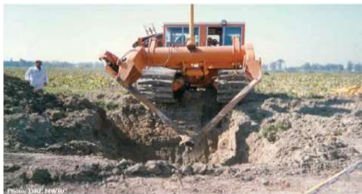
Figure 3. V-plough trenchless drainage machine
