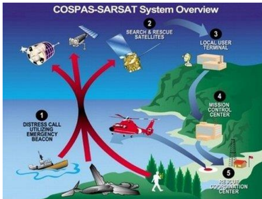
Figure 2 shows an overview of COSPAS-SARSAT System (Source: “COSPAS-SARSAT”, 2019).
