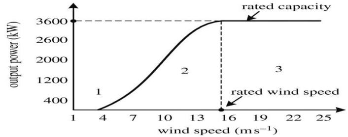
Fig-: 2Graph b/w output power & wind speed (VAWT)
