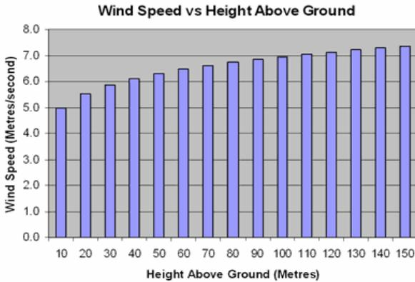
Fig:- 4Graph b/w wind speed & Height above ground
