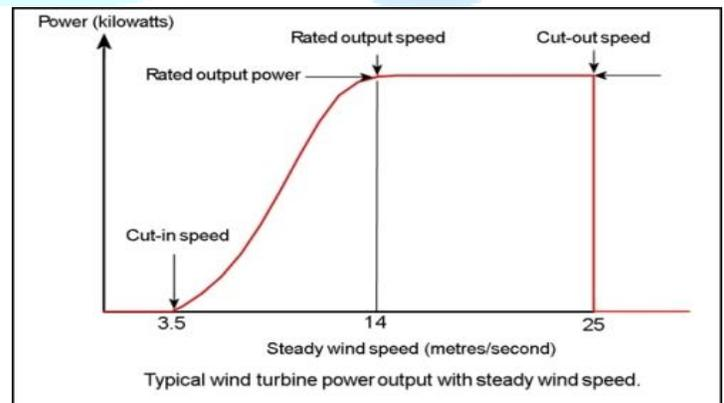
Fig-:3Required wind speed rotate (vawt)
